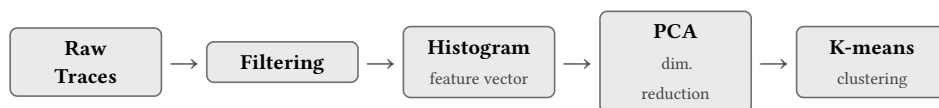
Figure 2.5: The four-stage analysis pipeline from our prior work: raw traces are filtered, encoded as conductance histograms, reduced by PCA, and finally partitioned by K-means.
